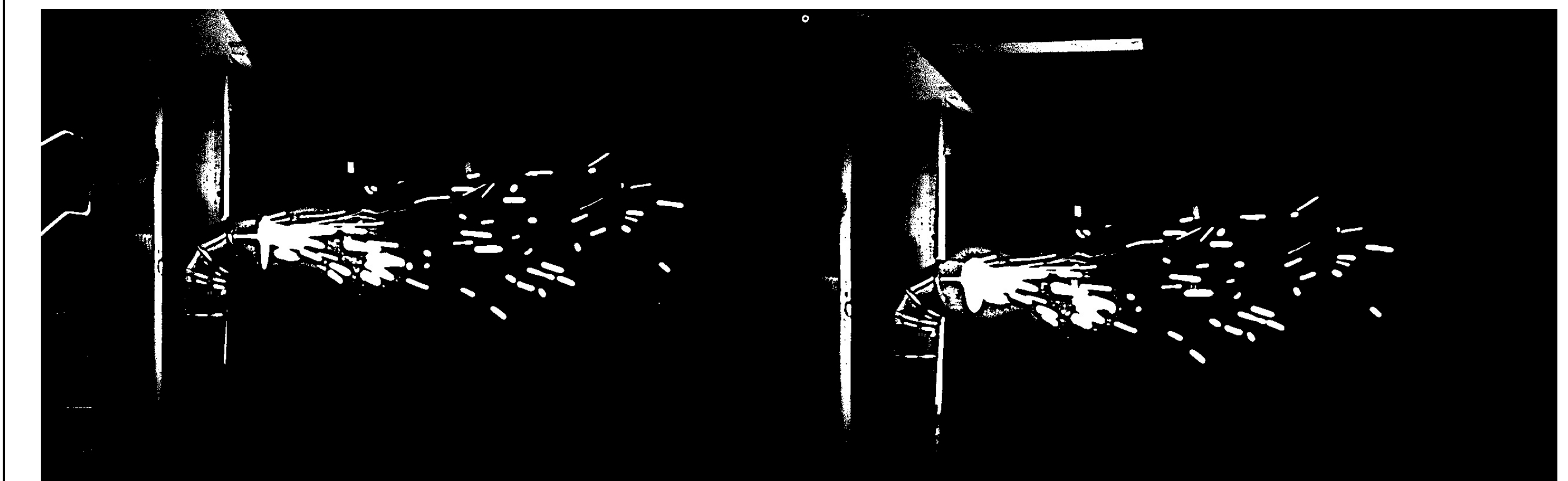
Figure 5. Preprocessed frames of footage from a firebrand simulation test, taken simultaneously with the two cameras.
