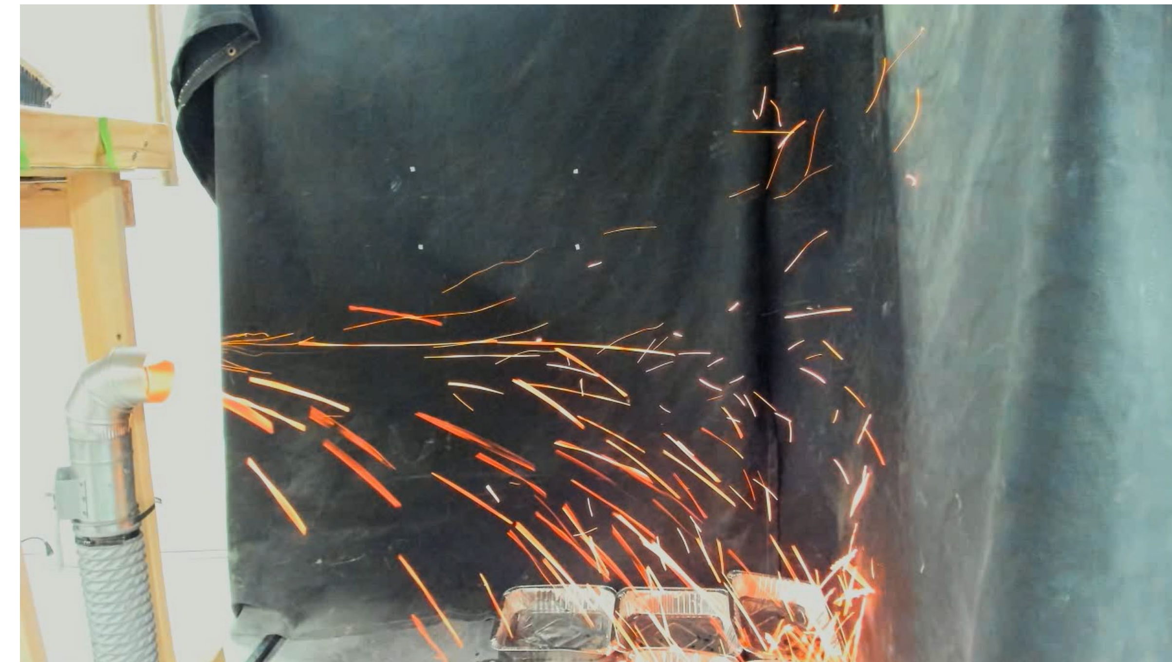
Figure 3. Firebrands lofting from the apparatus against a dark background for testing. The firebrands are produced by burning wooden dowels then loading into the apparatus.
