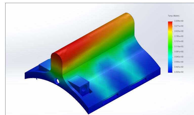
Fig 4. Thermal test on the spring housing
