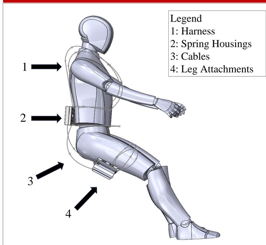
Fig 1. Model of our current prototype design produced in SolidWorks
