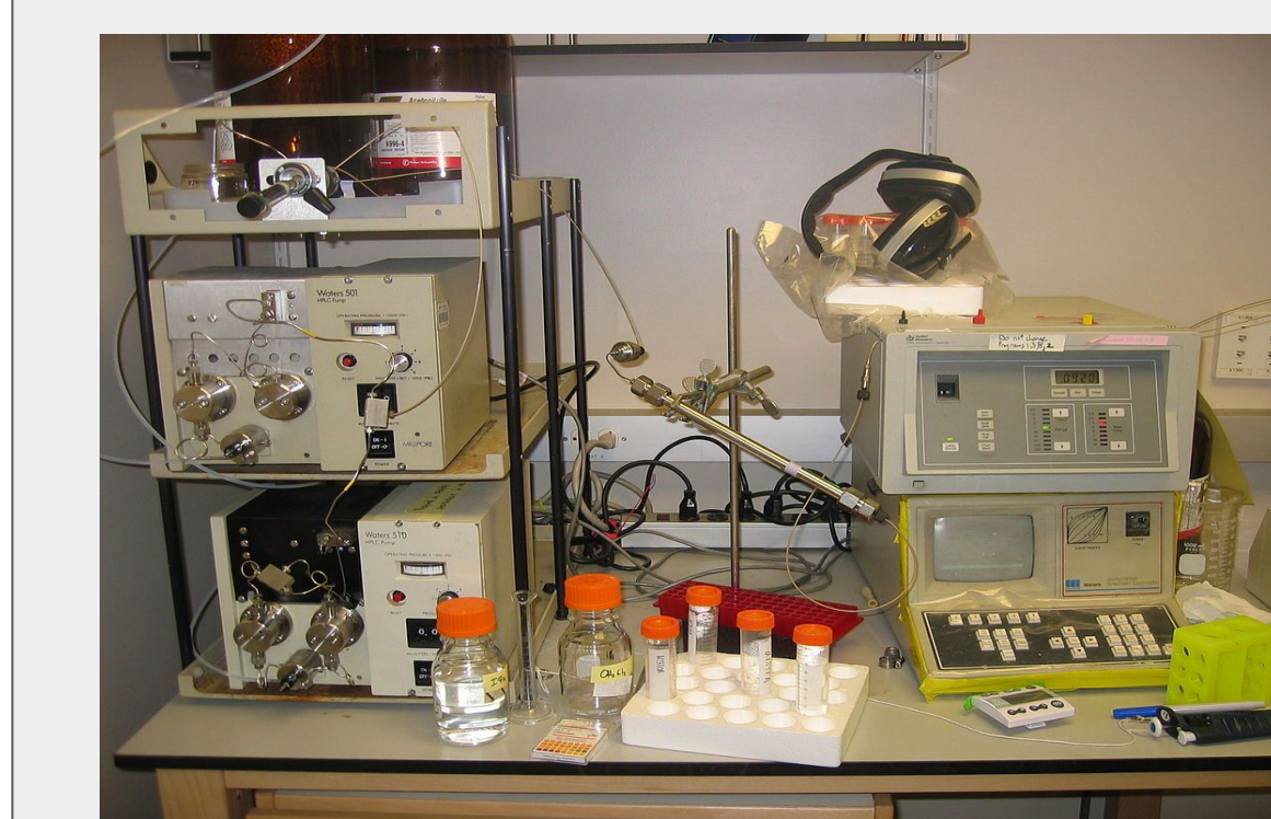
Figure 11a. Example of the setup for an HPLC in a laboratory setting
