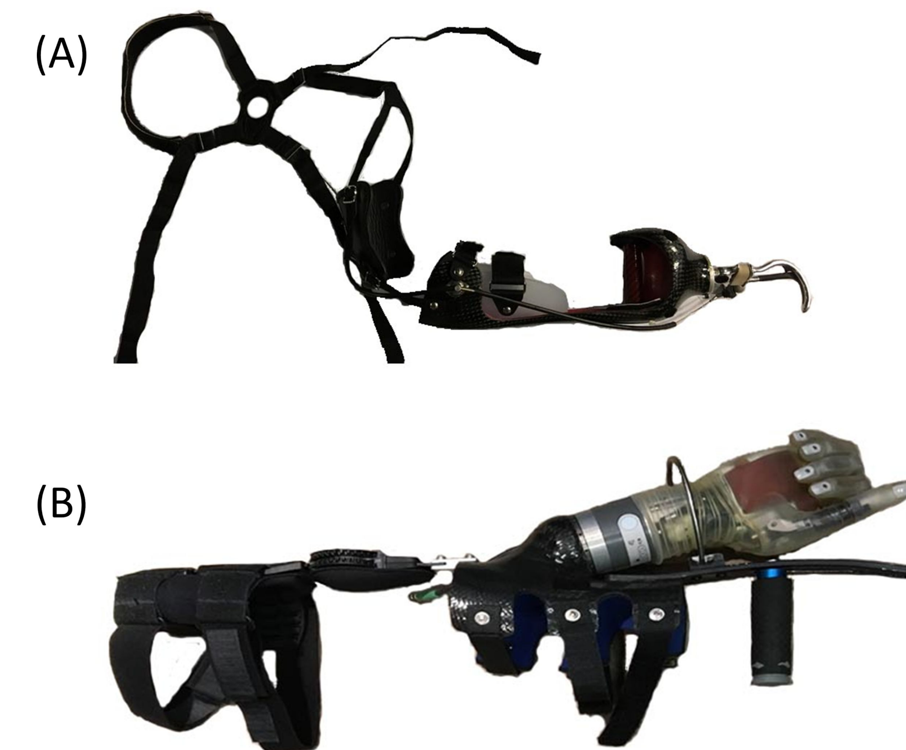
Figure 2. A) a body-powered prosthesis and B) a myoelectric bypass prosthesis. From "Application of machine learning to the identification of joint degrees of freedom involved in abnormal movement during upper limb prosthesis use," by Wang, S. L., Bloomer, C., Civillico, G., & Kontson, K., 2021
