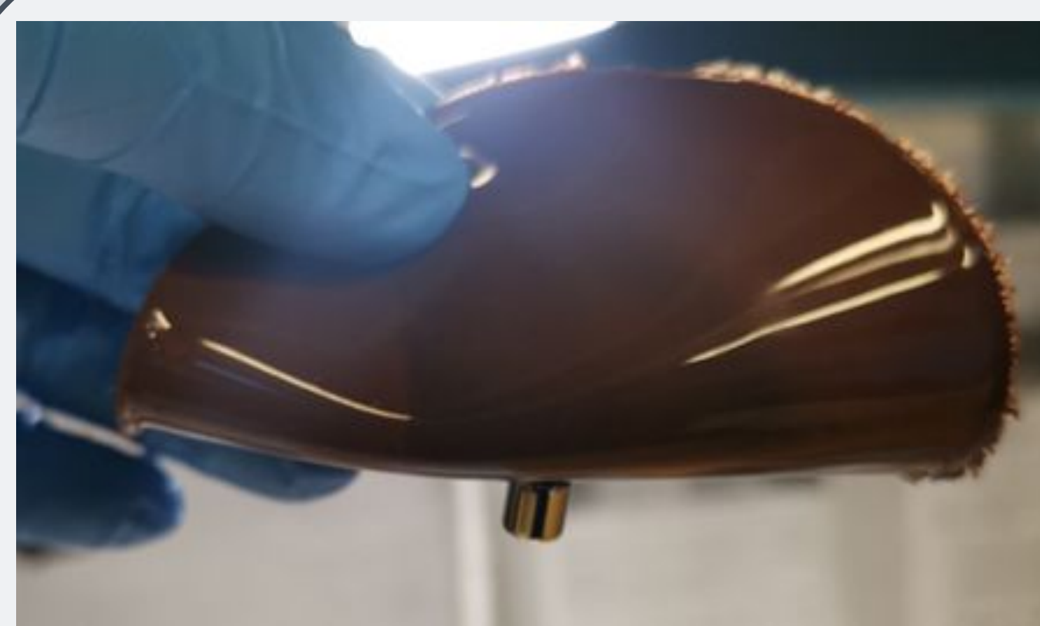
Figure 1: Photograph of a film fabricated using a preliminary ink of PDMS and \text{Fe}_3\text{O}_4 NPs
